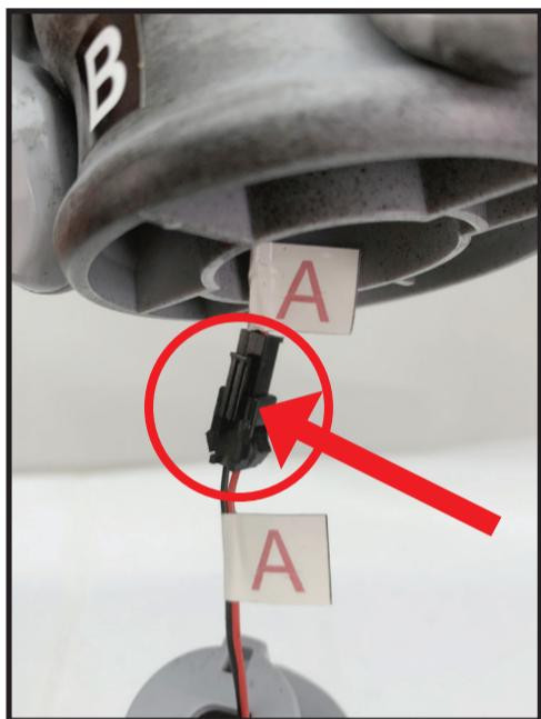
1. Attach wires from the SKULL labeled A to the wires from the POST labeled A.
